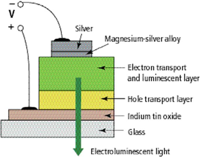
Figure 2: General diagram of an OLED8
